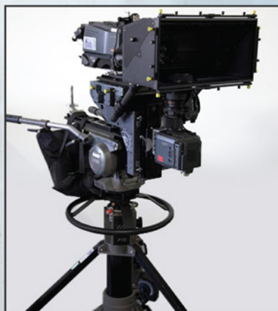
Stereoscopic 3D Rigs / Mounts using Panasonic, Sony and RED cameras and recorders
